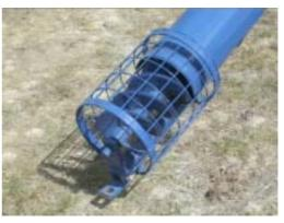
A problem with auger guarding *risk control* is that existing auger guards do not meet the Australian Standard for machinery guarding, and cannot meet Australian Standards and still operate effectively (see the dimensions in the *Guarding Advice* section above.
