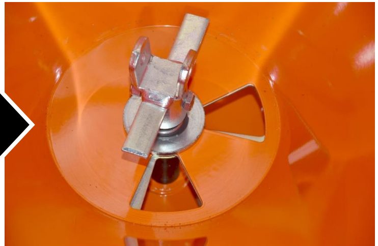
Direction shutter set to disperse material to both sides
