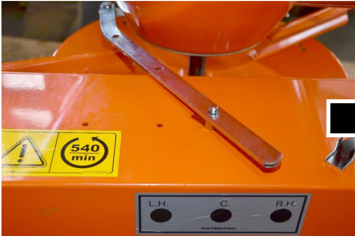
Direction shutter set to disperse material to the right hand side
