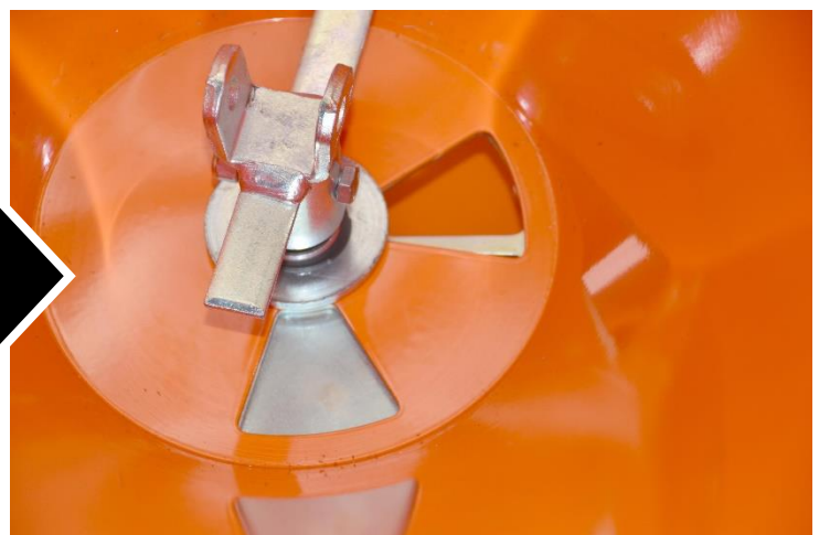
Direction shutter set to disperse material to the left hand side
