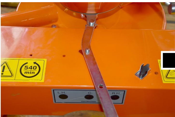
Direction shutter set to disperse material to the left hand side
