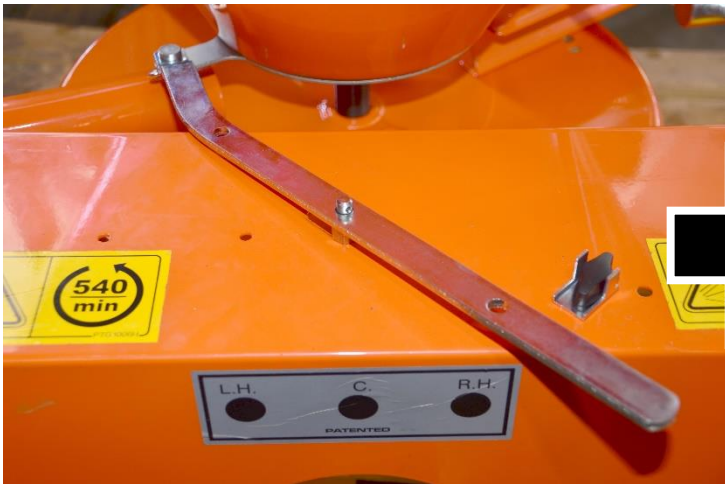
Direction shutter set to disperse material to both sides
