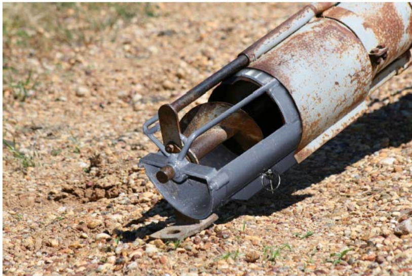
Old auger with inner guard retrofitted
