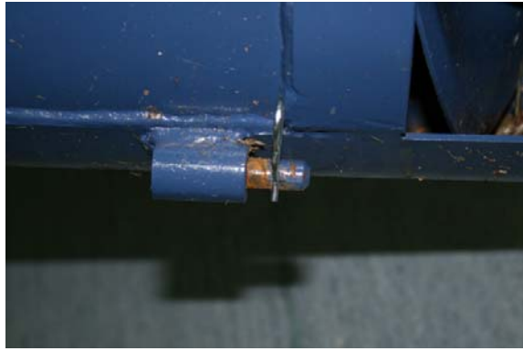
Detail of lug and pin to attach outer guard
