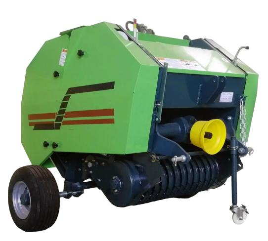
The 700mm Mini Round Baler makes baling a breeze. Aim to have your windrows at 800mm wide, optimal for pickup. This unit features dual twine spools plus electric alarm and bale ejection control, which is easily passed through to the tractor.
