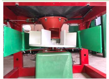
Green flaps (left and right) are adjustable. Use wing nuts to tighten.
