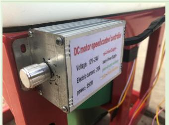
DC motor speed controller, controls speed of spinner.
