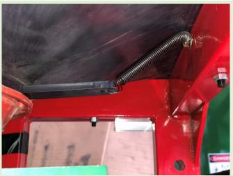
Ensure spring is attached to longer fertiliser gate tab as shown.
