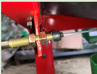
Attach control cable mount to welded tab on spreader frame as shown.
