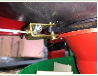
Attach control cable to shorter fertiliser gate tab as shown.
