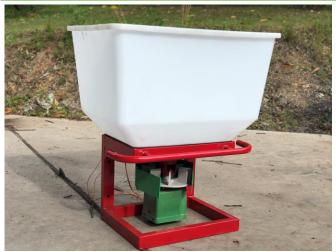
Attach hopper to frame as shown
